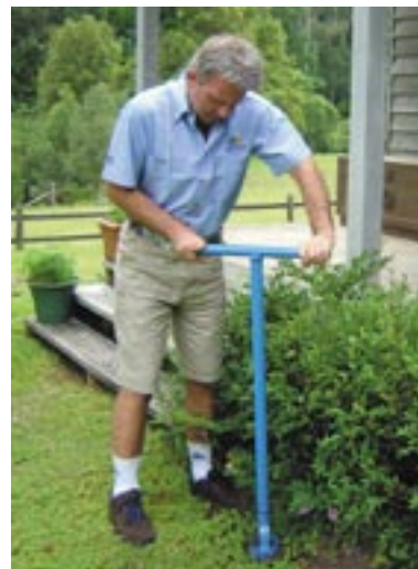
Using auger to place Exterra Station.
